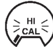
**Note:** Ensure that the CAL knob is not pressed as this will put the instrument back into calibration mode and the unit will need to be re-calibrated.
