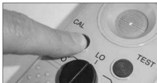
In case an oil of another brand is checked, recalibration of the instrument will be needed.
